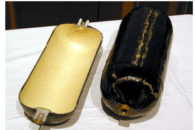
Super Pressure Hydrogen Gas Tank Using Liquid Polymer Liner (Fuji Heavy Industries. Ltd. )
