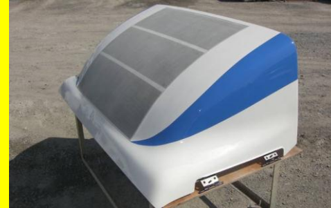
Air deflector for vehicles with flexible solar cell
